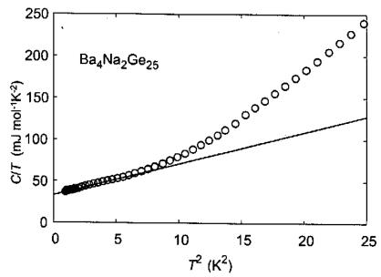
The graph above shows the heat capacity per mole of the metallic compound  $Ba_4Na_2Ge_{25}$ , measured to 5 K and plotted as C/T vs.  $T^2$ . The line is a linear fit to the low-temperature region. The molar volume of  $Ba_4Na_2Ge_{25}$  is  $V_m = 4.6 \cdot 10^{-4}$  m<sup>3</sup>.
