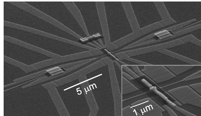
*A SAW driven electron interferometer*
