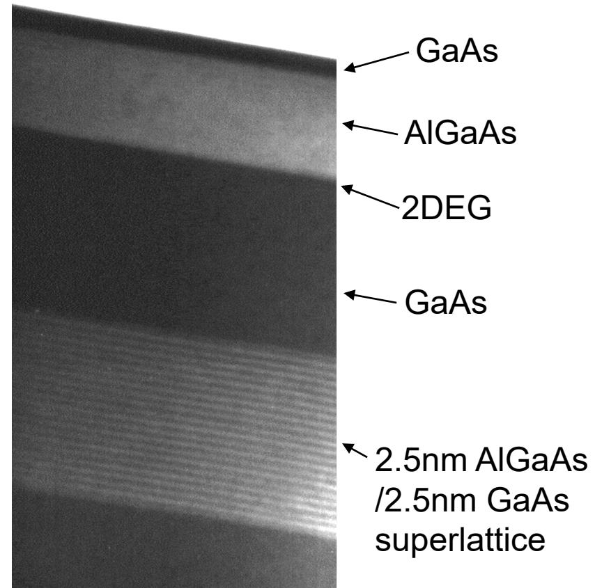
TEM of GaAs/AlGaAs 2DEG structure with superlattice buffer (W M Stobbs, Materials Science)
