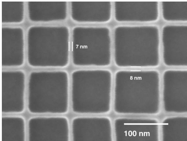
*A micrograph of a grid formed in ZnO demonstrating a sub-10nm resolution*
