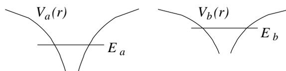
Figure 3.3: A simple model of a diatomic molecule. The atomic Hamiltonian is  $H_i = T + V_i(r)$ , with  $T$  the kinetic energy  $-\hbar^2 \nabla^2 / 2m$  and  $V_i$  the potential. We keep just one energy level on each atom.
