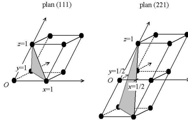
Figure 3.7: Definition of lattice planes and Miller indices. If a plane intersects the axes at  $x\mathbf{a}_1$ ,  $y\mathbf{a}_2$  and  $z\mathbf{a}_3$ , then the Miller index  $(hkl)$  is given by the smallest set of values  $h, k, l$  for which  $hx = ky = lz = \text{integer}$ .
