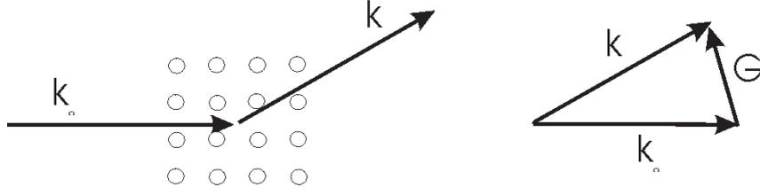
Figure 3.8: Illustration of Bragg scattering from a crystal
