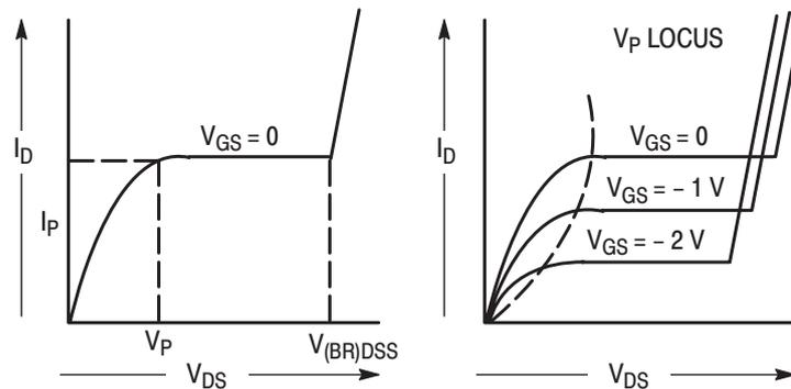
Figure 8.15: Current voltage characteristics of an  $n$ -type JFET with  $p$ -type gate. With increasing drain-source voltage  $V_{DS}$ , at constant gate-source voltage  $V_{GS}$ , the drain-source current  $I_D$  first rises roughly linearly. Pinch-off causes it to saturate at a level ( $I_P$ ), which depends on  $V_{GS}$ .
