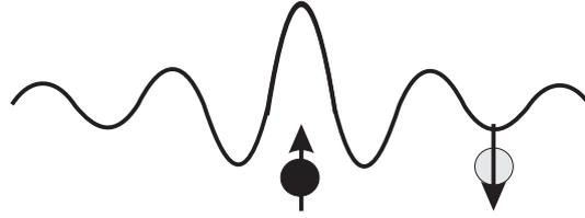
Figure 9.11: In metals, a local moment will polarise the conduction electron spins, producing a spin density that decays with distance and oscillates in sign with period  $1/2k_F$ . The interaction of the induced spin density with a neighbouring local moment produces the RKKY interaction.
