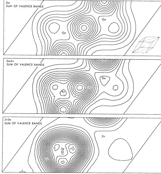
Figure 5.8: The valence charge density for Ge, GaAs, and ZnSe from an early pseudopotential calculation, plotted along a surface in a 110 plane that contains the two atoms of the unit cell. Note the (pseudo-)charge density shifting from the centre of the bond in Ge to be almost entirely ionic in ZnSe. [M.L. Cohen, *Science* **179**, 1189 (1973).]
