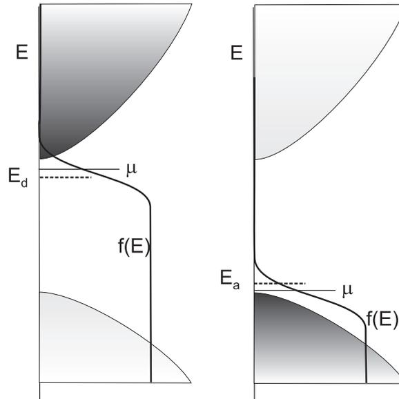
Figure 7.3: The left hand figure shows the effect of donor levels at an energy  $E_d = E_c - \Delta_d$ . The chemical potential will shift to near the conduction band edge, increasing the electron density and decreasing the hole density in comparison to the intrinsic case, while the product of the two is nevertheless constant. The right hand figure shows the corresponding picture for acceptor levels at an energy  $E_a = E_v + \Delta_a$ .
