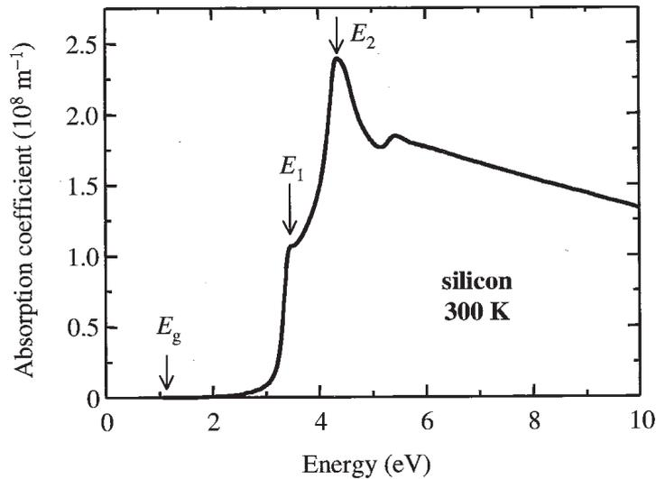
Figure 6.2: The interband absorption spectrum of Si has a threshold at the indirect gap  $E_g \approx 1.1 \text{ eV}$  which involves a phonon and is very weak. The energies  $E_1$  and  $E_2$  correspond to critical points where the conduction and valence bands are vertically parallel to one another; absorption is direct (more efficient) and also enhanced by the enhanced joint density of electron and hole states. [E.D. Palik, *Handbook of the optical constants of solids*, AP, 1985]
