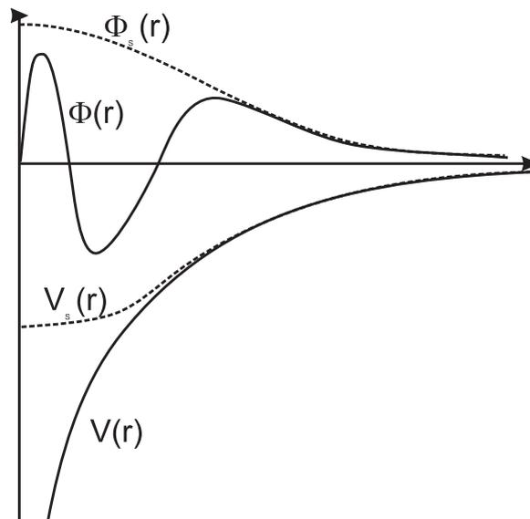
Figure 4.7: Pseudopotential: The true potential  $V(r)$  has a wavefunction for the valence electrons that oscillates rapidly near the core. The pseudopotential  $V_s(r)$  has a wavefunction  $\Phi_s(r)$  that is smooth near the core, but approximates the true wavefunction far from the core region.
