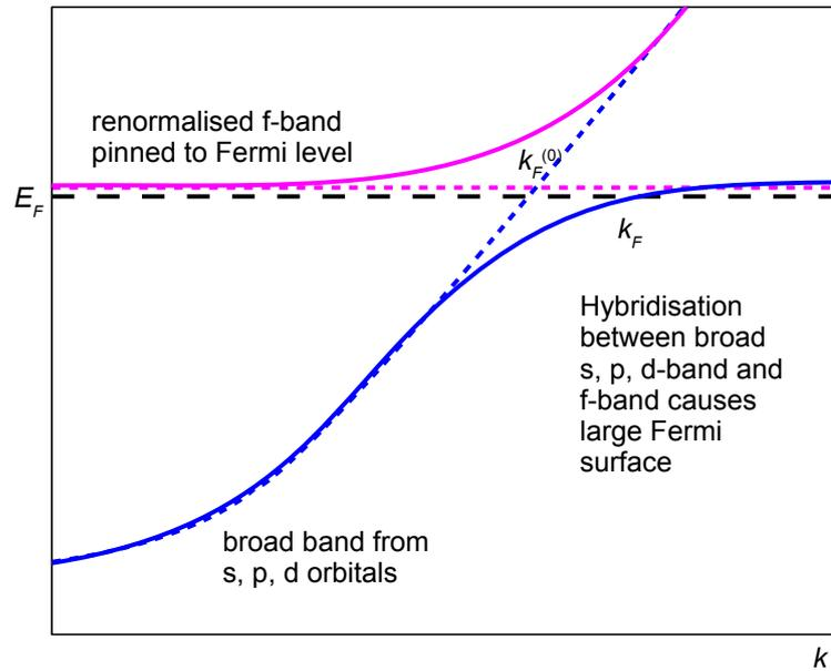
Figure 10.10: Schematic band structure for heavy fermion materials
