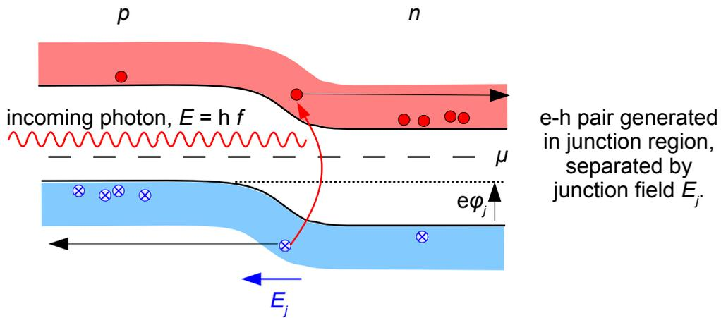
Figure 8.9: Operation of a  $p$ - $n$  junction based solar cell. When illuminated, electron-hole pairs are generated. Pairs generated away from the junction will recombine rapidly, but those electrons and holes generated near the junction will be separated by the in-built electric field. Electrons flow towards the  $n$ -side, holes towards the  $p$ -side, which is equivalent to increasing the generation current, which flows in the reverse direction ( $n$  to  $p$ ).
