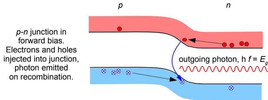
Figure 8.13: Principle of operation of a light emitting diode (LED).
