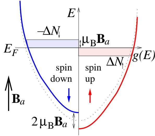
Figure 9.10: Effect of an applied field  $B_a = \mu_0 H$  on the spin-up and spin-down electrons in a metal. The spin-dependent shift of the energy levels – while keeping the chemical potential (and the Fermi energy) constant – produces a population imbalance between the two spin species. This converts to a magnetic moment, which is proportional to the density of states at the Fermi level.
