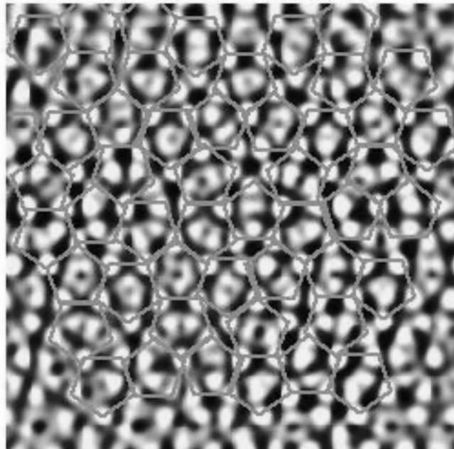
Figure 3.5: Scanning tunnelling microscope image of a 10 nm<sup>2</sup> quasicrystal of *AlPdMn* with a Penrose tiling overlaid. [Ledieu et al. Phys.Rev.B **66**, 184207 (2002)]
