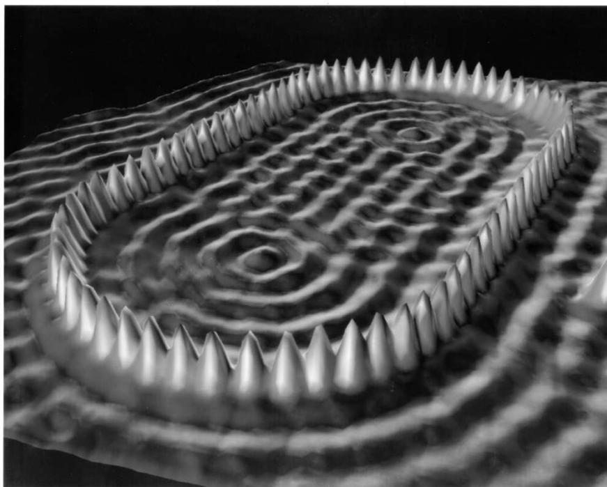
Figure 6.10: An array of Fe atoms arranged in a corral on the surface of Cu traps a surface electron state whose density can be imaged by STM. M.F. Crommie, C.P. Lutz, D.M. Eigler, E.J. Heller. *Surface Review and Letters* 2 (1), 127-137 (1995).
