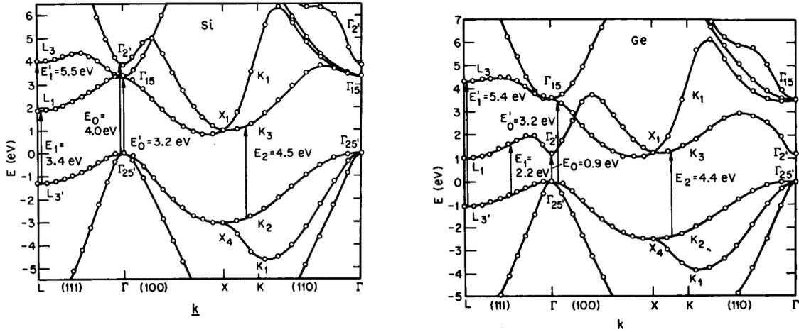
Figure 5.6: Pseudopotential band structure of Si and Ge [M.L. Cohen and T.K. Bergstresser *Phys. Rev.* **141**, 789 (1966)]. The energies of the optical transitions are taken from experiment.
