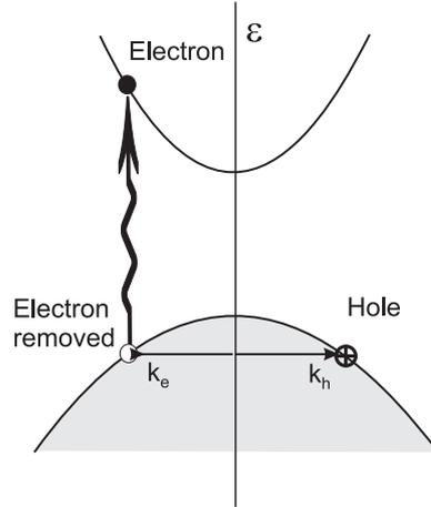
Figure 5.11: Absorption of a photon creates an electron-hole pair, with an energy  $\epsilon_e + \epsilon_h + 2E_{gap}$  but adds negligible momentum to the system. Hence the hole momentum is the negative of the momentum of the empty electronic state, and its energy is positive (measured conventionally from the top of the band).
