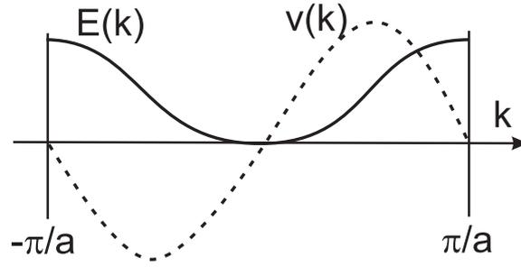
Figure 5.9: Band energy  $E(k)$  (solid line) and group velocity  $v(k)$  dashed line in a simple 1D band. A wavepacket progressing its crystal momentum according to (5.17) accelerates as  $k$  increases from zero, and then slows and reverses direction as  $k$  approaches the zone boundary.
