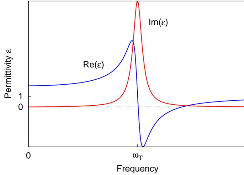
Figure 1.2: Real and imaginary part of the relative permittivity within the Lorentz (or dipole) oscillator model. Note that  $\epsilon = \chi + 1$  and the polarisability  $\chi_\omega$  has the frequency dependence typical for a damped harmonic oscillator.
