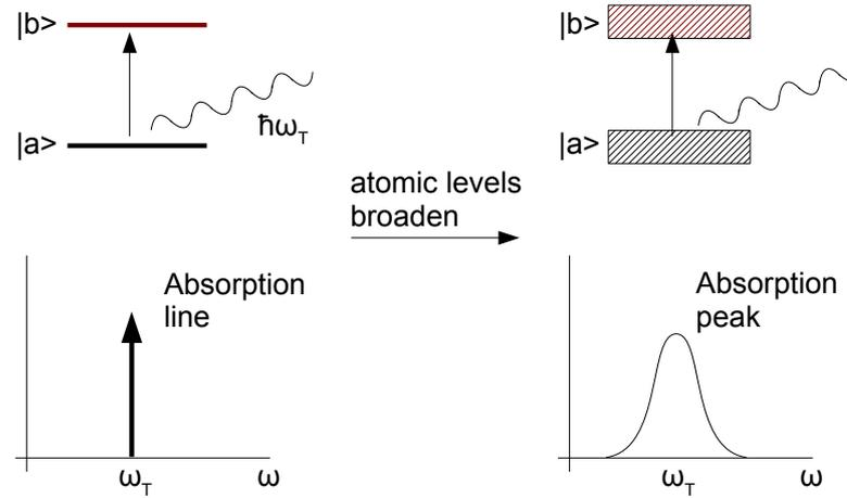
Figure 1.3: Absorption spectra produced by electronic transitions in atoms (discrete levels) and solids (levels are broadened). In solids, the sharp absorption peaks found in atomic spectra broaden out into resonances with a finite width. The resulting absorption spectra have a similar, Lorentzian form to that expected from the dipole oscillator model
