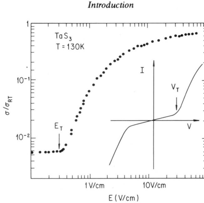
Figure 9.7: The inset shows the current induced in the cdw material  $TaS_3$ , and the main panel is the differential conductance  $\sigma = dI/dV$ . Below a threshold voltage, the CDW is pinned, and the only contribution to the current is the thermal activation of carriers across the CDW gap. Above  $V_T$ , there is a large contribution to the current that grows in a nonlinear fashion with increasing voltage, which is the contribution of the sliding of the CDW.[From Gruner and Gorkov,]
