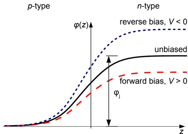
Figure 8.6: The effect of applying a bias voltage across a diode. The potential across the junction is decreased in forward bias (corresponding to a positive voltage  $V$  applied to the  $p$ -type side) and increased in reverse bias.
