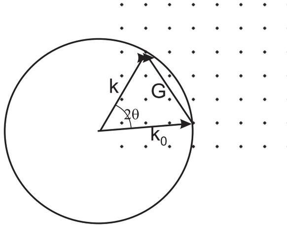
Figure 3.9: Ewald construction. The points are the reciprocal lattice of the crystal.  $k_0$  is the incident wavevector, with the origin chosen so that it terminates on a reciprocal lattice point. A sphere of radius  $|k_0|$  is drawn about the origin, and a diffracted beam will be formed if this sphere intersects any other point in the reciprocal lattice. The angle  $\theta$  is the Bragg angle of (3.21)
