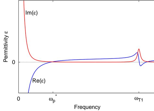
Figure 1.5: Real and imaginary part of the dielectric permittivity in the Drude model. The peak at  $\omega_{T1}$  illustrates the possibility of additional resonances due to the bound, core electrons.
