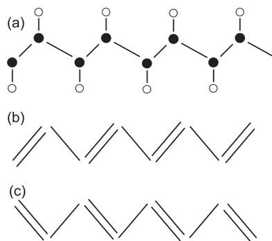
Figure 9.5: (a) shows a sketch of the atomic arrangement of polyacetylene, with the  $C$  atoms as solid circles, and the  $H$  atoms as open circles. The  $C$  atoms are not equally spaced, and the structure is often idealised as an alternation of “double” and ”single” bonds, (b) and (c). The two isomers in (b) and (c) are related by a mirror symmetry.
