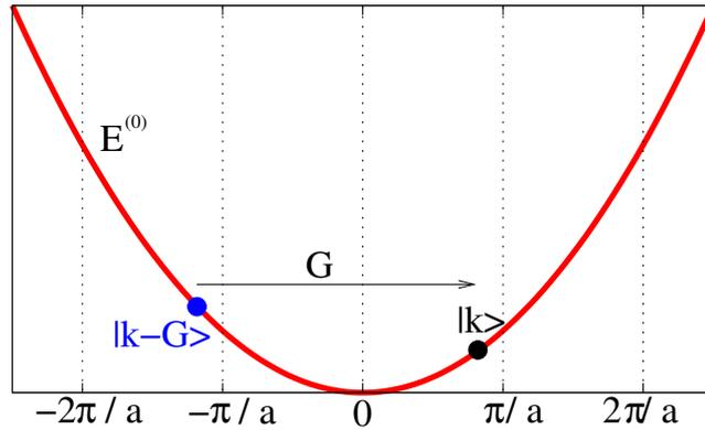
Figure 4.1: The nearly free electron approach illustrated for a one-dimensional solid. The first Brillouin zone boundary is at  $\pm\pi/a$ . States  $|k\rangle$  close to  $\pi/a$  are nearly degenerate with states  $|k - 2\pi/a\rangle$ , and the matrix element linking those states, the lowest Fourier coefficient of the lattice potential,  $V_{2\pi/a}$ , is non-zero. Hence, these two states mix (hybridise) to form the Bloch states near the Brillouin zone boundary.
