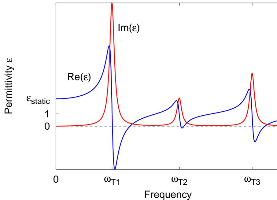
Figure 1.4: The electromagnetic response of an insulator can very generally be modelled by superimposing dipole oscillator responses with different natural frequencies, each scaled by a suitable oscillator strength. The low frequency, static permittivity then includes contributions from the low frequency tails of all the individual oscillator responses.
