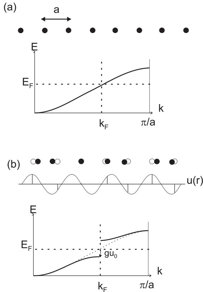
Figure 9.1: The Peierls transition. The upper figure shows the familiar one-dimensional chain with lattice constant  $a$  and the corresponding lowest electronic band, plotted for momenta between  $0$  and  $\pi/a$ . In the lower figure (b) a periodic lattice modulation is introduced, with  $u(r)$  of the form of (9.2). The period is cunningly chosen to be exactly  $2\pi/2k_F$ , so that a band gap of amplitude  $2g_Q u_0$  is introduced exactly at the chemical potential.
