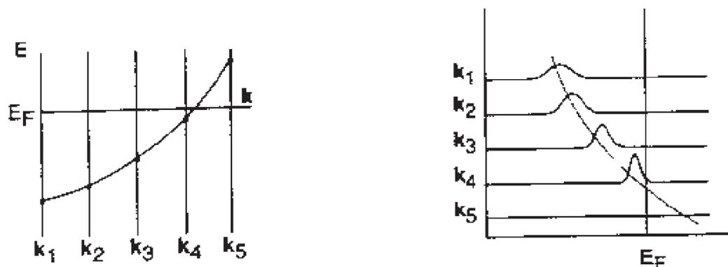
Figure 6.4: Idealised results from a photoemission experiment. A peak is observed at the band energy in each spectrum, but disappears when the band crosses the Fermi energy, where there are no more electrons to excite.
