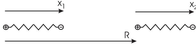
Figure 3.1: Two dipoles represent model atoms that are arranged along a line, with the positive charges (+e) fixed at the positions 0,  $R$ , and the negative charges ( $-e$ ) at the points  $x_1$ ,  $R + x_2$ .
