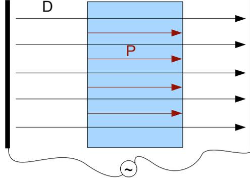
Figure 1.7: Exciting plasma oscillations by applying an oscillating electric field
